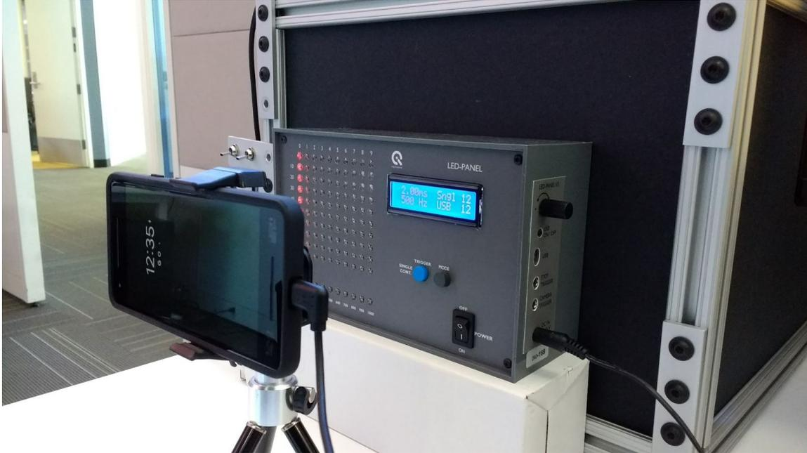
Figure 2(a): Side view of phone & LED tracer setup
