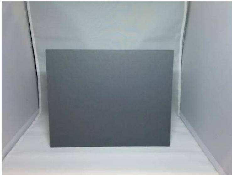
In particular, the grey card is roughly centered in the field of view, taking up around  $\frac{1}{2} \times \frac{1}{2}$  of the scene, with the white background visible on all sides around it. As is evident from the image above, a high degree of precision is not required; the most important factors are that the scene is completely static (including no light source flicker) and that the very center of the image is within the grey card area.
