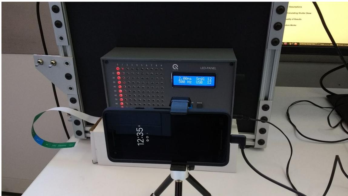
Figure 2(b): Front view of phone & LED tracer setup
