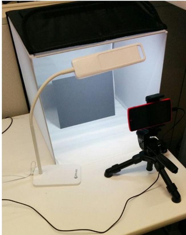
The desk lamp should be reasonably bright: bright enough that it wouldn't be considered a "low light" environment, but not so bright that the device's flash won't make any difference to the scene illumination when turned on. Using the specific desk lamp in this example, setting the brightness to the middle of its three adjustable brightness levels works well.
